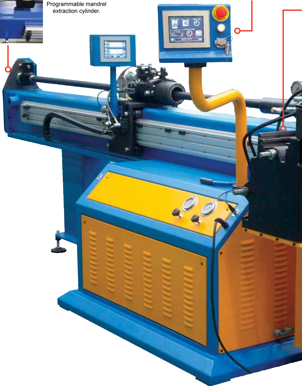
Touch screen with USB unlimited program storage.
